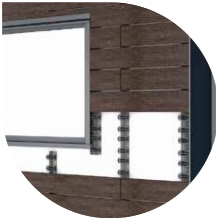
Demountable clip-system GRAD® system for MOSO® Bamboo Thermo Cladding
